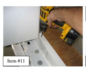
Attach the doorframe to the vehicle using #10 x 1" Phillips pan head sheet metal screws
